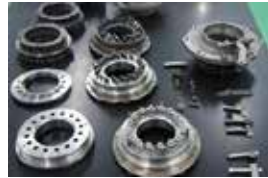
Disassembled variable nozzle. Each component is identified.
