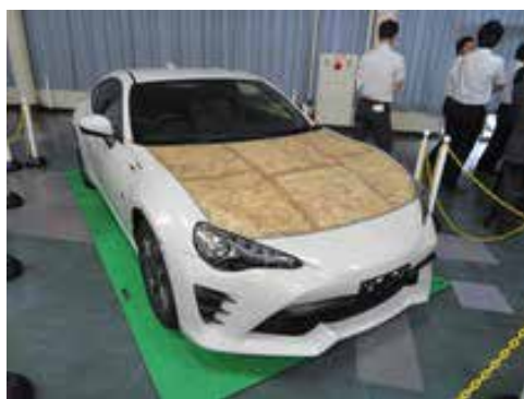
Toyota 86 fitted with CNF prototype parts. The car was produced by Toyota Customizing & Development Co., Ltd.
