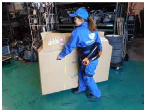
Ms. Nakanishi is fitted with HAL during packaging work. Even female workers can easily transport heavy goods.
