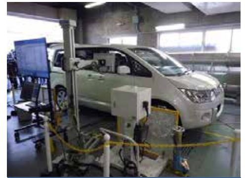
Measuring fuel economy and exhaust emissions from a vehicle
