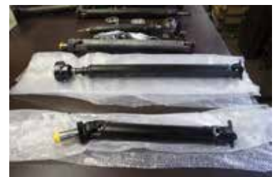
'Replace' propeller shaft is produced with the support from partner companies
